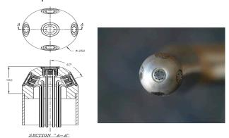
Figure 1: High Temperature 5-Hole Probe
