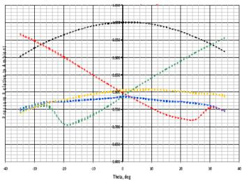
Figure 2: Pressure Reading as Function of Yaw Angle with Elevation Angle of 0 Degrees. Five runs show excellent overlap
